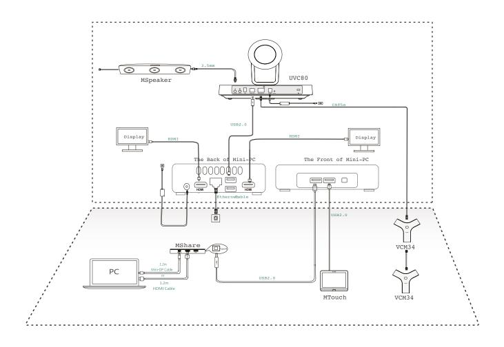
For convenience, we recommend that you connect a wireless USB dongle to the back of the Mini-PC to use mouse and keyboard to manage devices.
